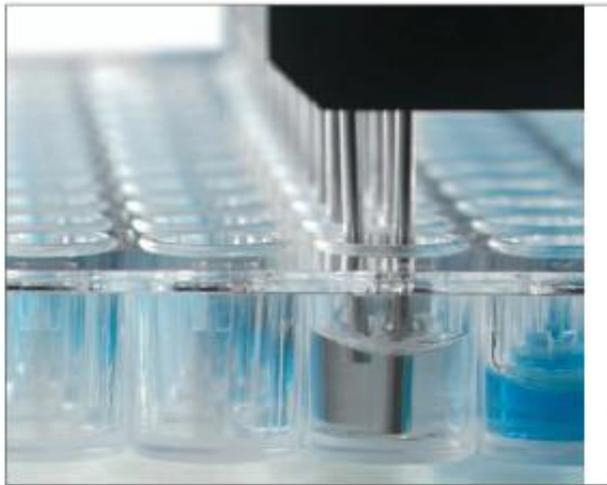
*Proper positions of manual washer needles for dispensing wash solution*
