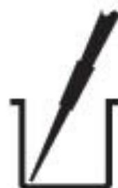
*Proper position to dispense reagents into empty wells using a multichannel pipette; in the lower corner of the wells*
